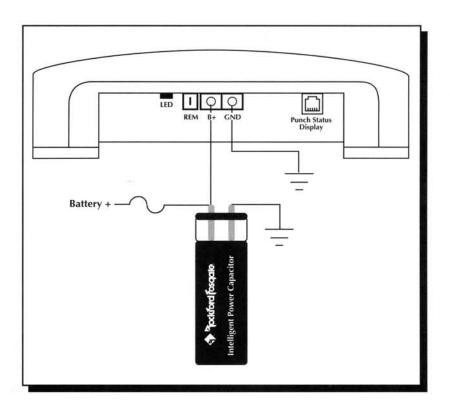
• Recommended capacitance is 1 farad per 1000 watts
