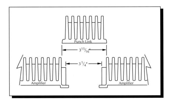
• Amplifier Spacing is  $3^{15}/_{16}$ " (10cm) between heatsink fins
