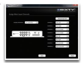
4. On the Assign Output Channels page the output channels can be assigned and named according to where they are located in the vehicle.
