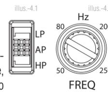
Placing the crossover switch in the AP position sets the amplifier to the All Pass mode, preventing any crossover adjustment, allowing all frequencies to pass.
