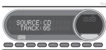
Note: Use the 40Hz @ 0dB tone (Track 5) for mono amplifier applications or the 1kHz @ 0dB tone (Track 7) for multi-channel amplifier applications. Be sure your x-over is switched to the appropriate filter setting.
