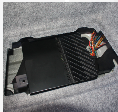
Fig. 3 - Premium factory installed systems use small external amplifiers.
