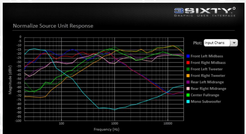
Fig. 5 - 3SIXTY.3 can sum multiple sources to create a full bandwidth output complete with fader control.
