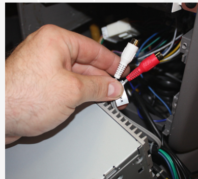
Fig. 1 - Radios with RCA jacks provide a low level signal for amplifiers.
