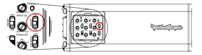
The PRESET switch disables the control panel and sets this amp for the best sound to be used with your ROCKFORD FOSGATE stage kit audio system. Turn the switch OFF to manually adjust this amp.
